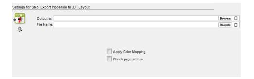
Apply Color Mapping: You can enable this to export the layout file with the same color mapping as defined in the Plates view.
